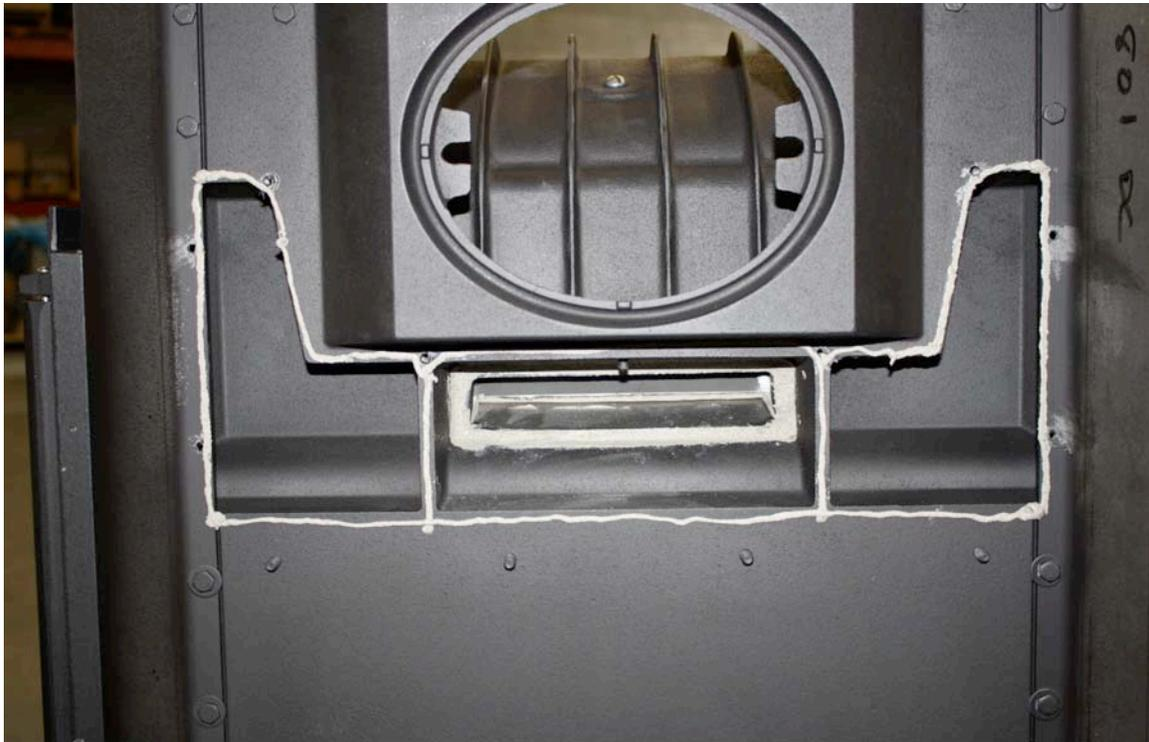
5. Use the four lower bolts as a guide to align the damper assembly with the back of the stove. Press the assembly into the cement evenly. Start the two outside nuts at the bottom corners. Start the two bolts at the upper corners. Start the remainder of the nuts and bolts.
